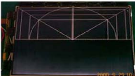
Horizontal Block Gate TAB IC Defect
