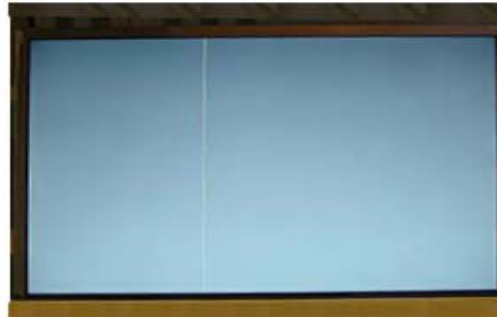
Vertical Line Source TAB IC Defect
