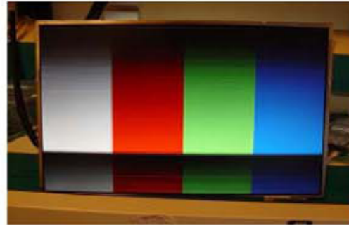
Horizontal Block Gate TAB IC Defect
