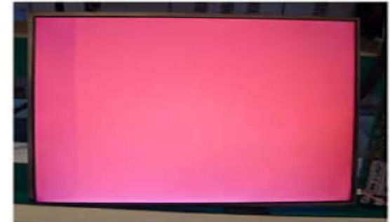
Vertical Block Source TAB IC Defect
