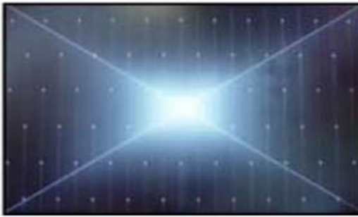
Solder defect, Short/Crack
