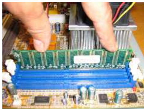
Figure 170 Insertion des barrettes DIMM
