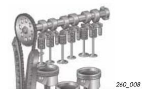
4-valve drive Bushed roller chain Camshaft sprockets Hydraulic chain tensioner Timing case Sprocket drive of camshafts and oil pump **Bushed** roller chain Spring-loaded chain tensioner 260\_002 260\_007 Oil pump sprocket Oil pump
